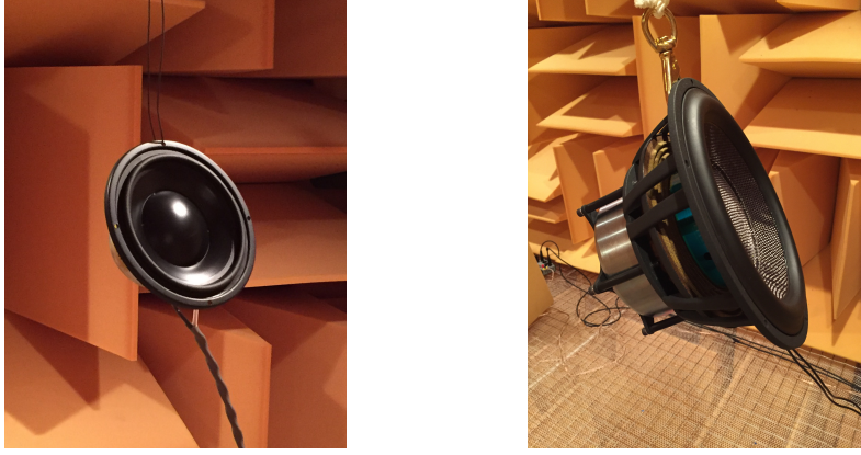
Figure 4. Tested drivers suspended in low-frequency anechoic chamber. Left: Morel MW-166es woofer, right: Morel UW-1058c subwoofer
